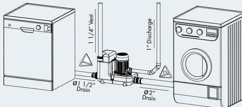
**Powerful 1 HP drain pump for commercial applications** where hot water can be an issue as it is capable of handling up to 194°F. System is capable of **handling multiple fixtures simultaneously**. Powerful motor for absolute reliability and efficiency.
