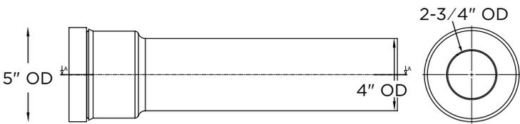
The 18" extension pipe was designed with the idea to simplify the installation process making it easier to **hide the pump and plumbing behind the wall**. It has an inner gasket which connects to the rear spigot of the Saniflo toilet creating a sealed connection.
